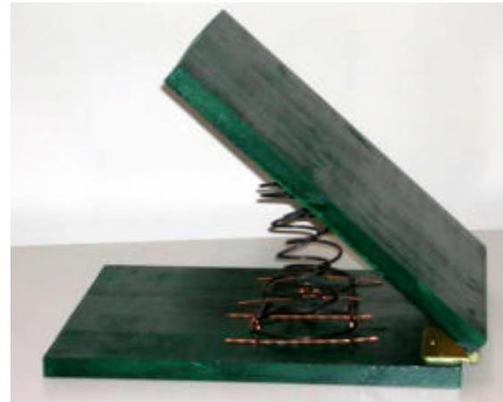
Figure 13. Photograph of the spring loaded chair seat prototype.
